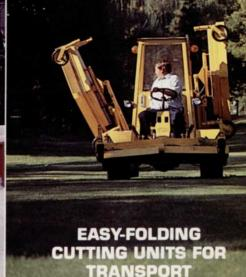
Your search for a high capacity mower encompassing a one man operation is now concluded. The Hydro-Power 180 with its 15 foot hydraulically driven rotary mower has a mowing capacity of up to 11 acres an hour while incorporating rear wheel steering for maximum maneuverability. Cutting units are designed for maximum floatation and may be used individually or in any combination of the three.
