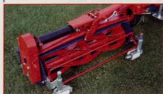
Fixed cutting unit, with anti-scalp rollers.
