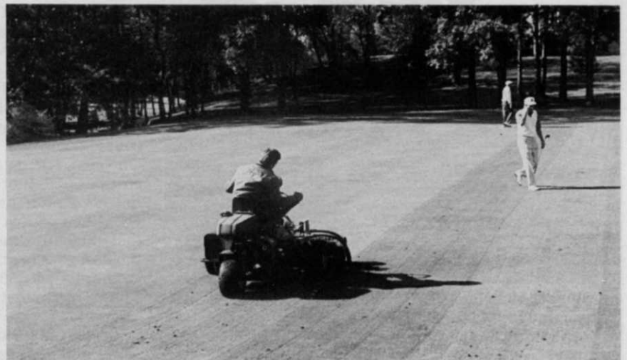
McBride is a firm believer in verticutting. In preparation for triplex mowing, an operator uses a greens verticutter on the 10th fairway without interfering with the golfers.
