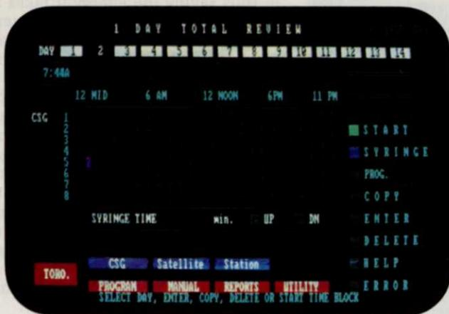
*This screen quickly displays complete irrigation program for one full day, for each of 14 days in the system.*
