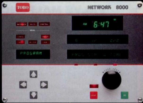
Matching the Network 8000 central for advanced and innovative design is Toro's new satellite/stand-alone solid state controller. It is a 32-station unit, with each station capable of operating three Toro electric valve-in-head solenoids.
