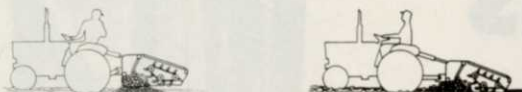
Open bottom—PTO Drive. Rocks are raked to a convenient windrow for later pickup.
