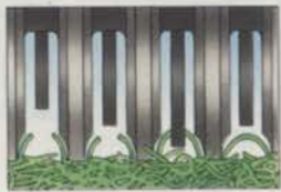
The knife blades rotate through slots in the front rollers, slicing horizontal runners before they lie down.
