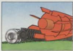
The horizontal reel follows closely behind to clip grass while it's standing straight, for faster, truer greens without lowering height of cut.
