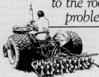
The Ryan Tracaire — built specifically for athletic fields and other flat grounds.
