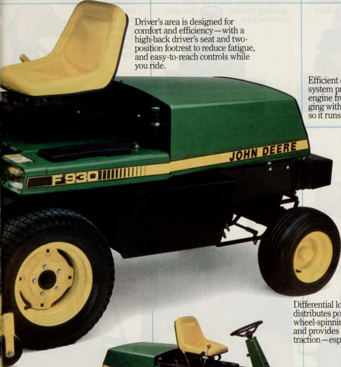
Driver's area is designed for comfort and efficiency — with a high-back driver's seat and two-position footrest to reduce fatigue, and easy-to-reach controls while you ride.
