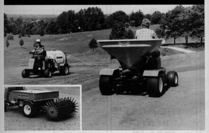
Greens or fairways ... the Multi-Pro 44 with its big high flotation tire to protect your turf, converts in minutes to a Sprayer, Spreader, Aerifier or Utility Bed. Designed for easy on, easy off switching and year 'round service.
