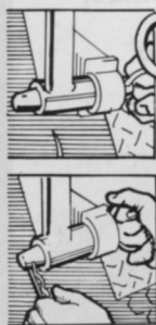
The exclusive Cushman pin disconnect system lets you attach and remove accessories in minutes.
