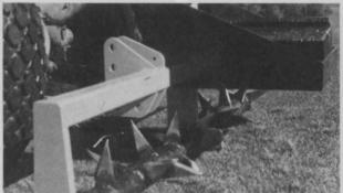
The AER-WAY is a low maintenance, low energy aerifier designed especially for hard, compacted traffic and playing areas and sod estab-lishment. The tines are 7" long and the unique, patented design fractures the soil between the tines enhancing the soil profile and its natural capillary action. This allows air, moisture and fertilizer to get to the root system promoting maximum growth and producing thicker, greener turf. And you save on fertilizer and irrigation usage.
