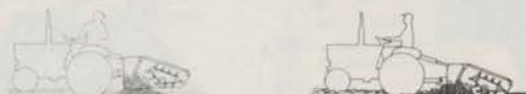
Open bottom—PTO Drive. Rocks are raked to a convenient windrow for later pickup.
