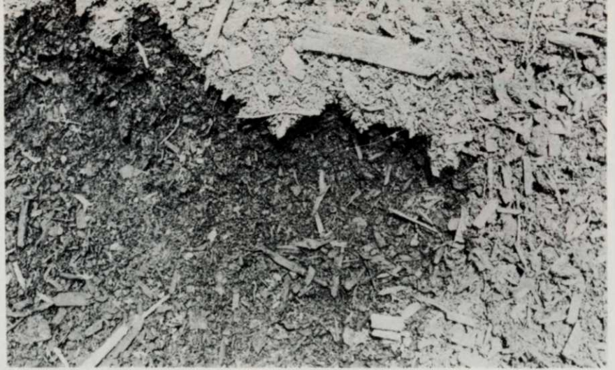
Wood chips are mixed with sludge for composting, then removed for spreading.
