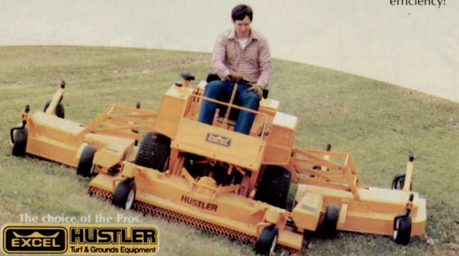
An automatic clutch on each wing disengages blades when wing is raised.
