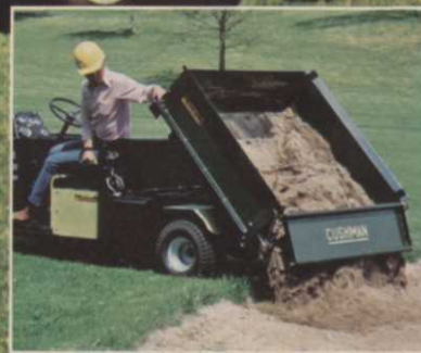
FLATBED BOX & SHORT BOX The Flatbed Box and Short Box attachments haul and dump 1500 pounds of sand or soil, with optional live hydraulics.
