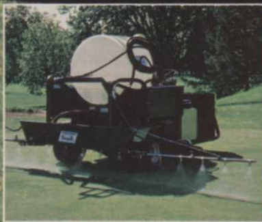
SPRAYER The Sprayer attachment sprays chemicals through an optional 15' rearboom or optional handgun.
