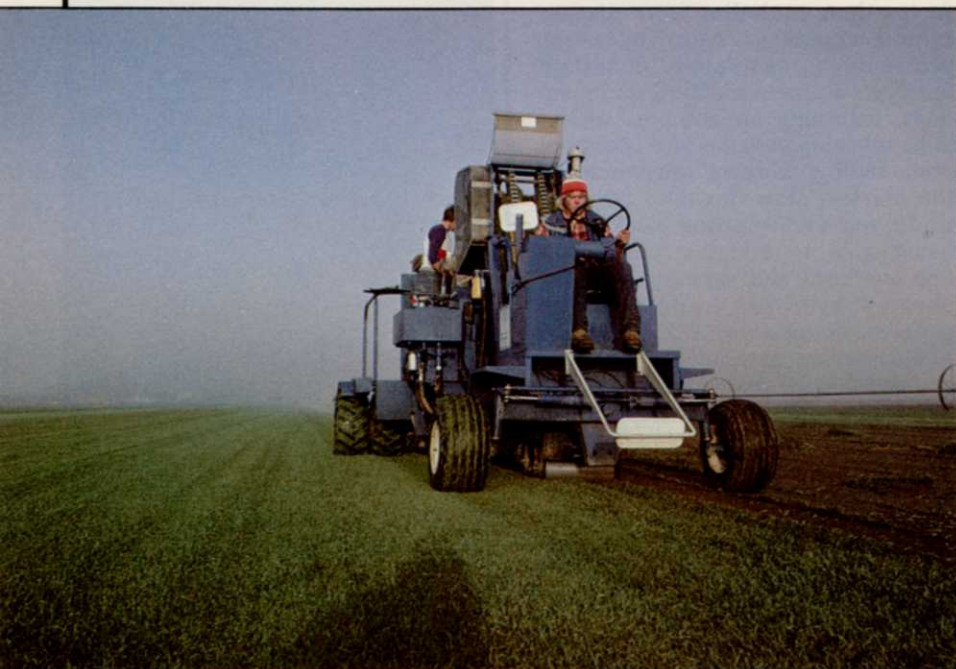
Modern sod equipment (Princeton harvester shown) increases speed and reduces handling.
