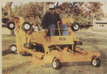
An automatic clutch on each wing disengages blades when wing is raised.
