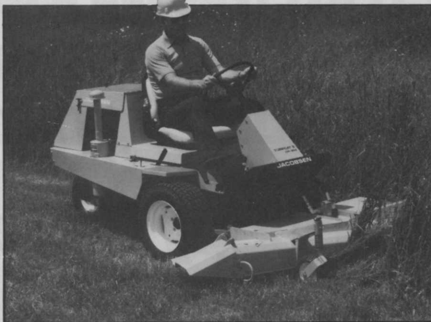
This riding mower's hydraulically driven cutter blades make short work of field grass. A snowthrower, dozer blade or rotary broom can be attached in place of the cutter deck to handle other chores throughout the year.
