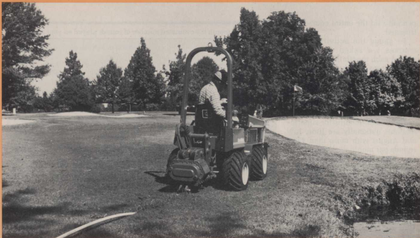
The Ditch Witch 350SX, a 35-HP-class lawn plow that's compact enough to go through a 36-inch gate.
