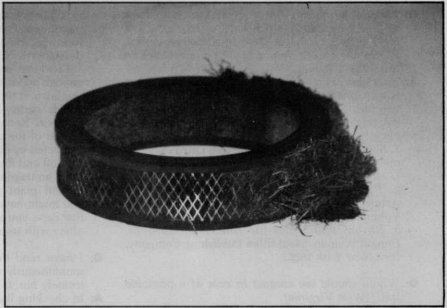
Due to dust, seeds, grass clippings, etc. attention to air cleaners is particularly important in summer months.
