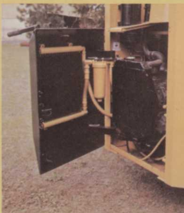
Swing-out rear door opens for easy servicing access.
