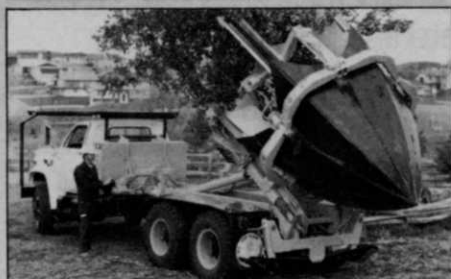
TS-84T. Truck-mounted. Transplants trees with maximum trunk diameter of 8". Six hydraulically activated, high tensile steel spades. Gravity-feed water tanks for spade lubrication.
