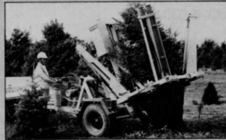
TS-44. Available in trailer-mounted, tractor-mounted or truck-mounted models. (Plus the option to extend or side shift for greater maneuverability as a truck-mounted unit.) Hydraulically transplants 4" diameter trees.
