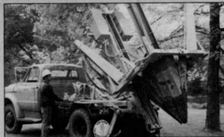
TS-50M. Truck-mounted. Outstanding maneuverability. Extension and side-shift features let you hydraulically position the spade an additional 21" away from the frame and 15½" left or right of center.
