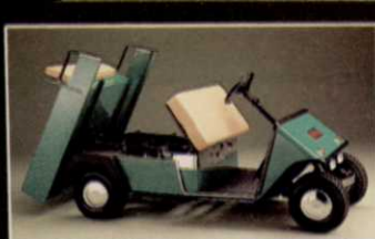
The load bed tilts for easy access to the drive package.
