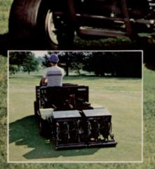
The Quick Aerator's 46" swath covers wide expanses of turf quickly. Choice of 3 tine styles: coring, slicing, open
