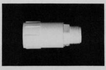
**King Brothers** has developed a device to prevent the theft of valuable sprinkler heads. The plastic Head-Lok fits between the riser and the sprinkler head below grade and swivels when vandals try to remove the head from above ground. The Head-Lok comes in  $\frac{1}{2}$ -in..  $\frac{3}{4}$ -in. and 1-in. sizes.
