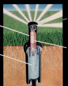
Nozzles seal when retracted
