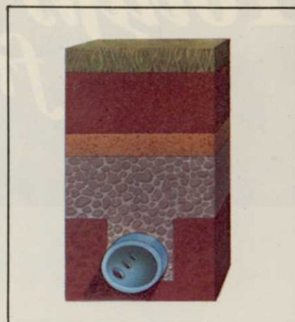
The drainage tile is inset in four-inches of pea gravel, which is then covered with a layer of coarse sand and a foot of topsoil.
