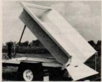
which can be operated by an individual standing at the rear of the unit through a 15 foot cable. The 14-gauge steel body has a 73 cubic foot capacity and can lift up to 6,000 lbs.
