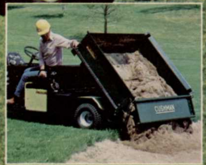
FLATBED BOX & SHORT BOX The Flatbed Box and Short Box attachments haul and dump 1800 pounds of sand or soil, with optional live hydraulics.
