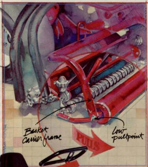
low pullpoints, that pulls rather than pushes. Resulting in balanced, fully floating cutting heads that allow the reels to float freely as they cut, unaffected by dips or bumps encountered by other parts of the machine. Or by the weight of clippings in the baskets.
