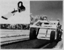
tools come with cutting edges of hardened steel or a tungsten carbide insert. Tools are tapped into holders and held in place by a compression cord wedged between each tool and holder.
