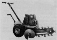
ly replaced hardfaced blades and a screw conveyor to deposit cuttings at the side of the trench. The trencher is compact and easy to operate and has four engine options available.
