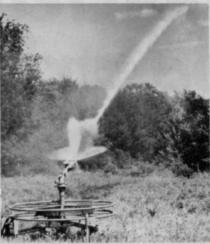
pressure of 65 psi. The trailer mounted unit measures six ft. by eight ft., weighs 325 lb., and has a 3-point trailer hitch base and horizontally mounted hose storage reel. It can irrigate an acre of land with one inch of water in three hours.
