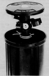
short radius stream and low application rates to resist runoff and puddling. Side and bottom inlets are ½ in., popup heights is 3 in. and throw range is 14 ft. to 23 ft. A multi-function wiper seal flushes, seals and wipes the pop-up stem.
