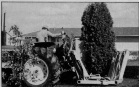
TS-30. Trailer-mounted or tractor-mounted. Ideal for nurseries, tree farms, rental yards and tree service firms. Adjustable towers enable operators to transplant or package either cone shaped or flat-bottom trees or shrubs up to 3" in diameter.
