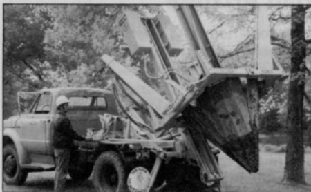
TS-50M. Truck-mounted. Outstanding maneuverability. Extension and side-shift features let you hydraulically position the spade an additional 21" away from the frame and 15½" left or right of center.
