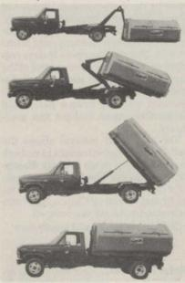
changeable container system may be used on a truck chassis of 10,000 pounds gross vehicle weight. Demounting of the container, lifting up, and dumping is accomplished in less than 30 seconds from inside the truck cab via remote control.
