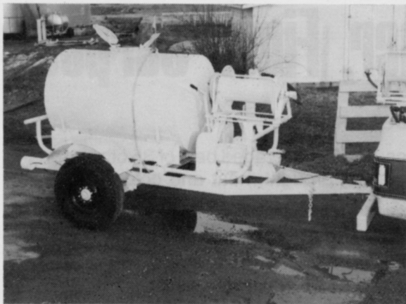
A 320-gallon lawn and tree care spray system by Westheffer has an electric start 8-hp gasoline engine.
