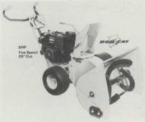
and reverse speeds without clutching. A rugged impeller rather than a fan discharges snow, which prevents plugging of the discharge chute.
