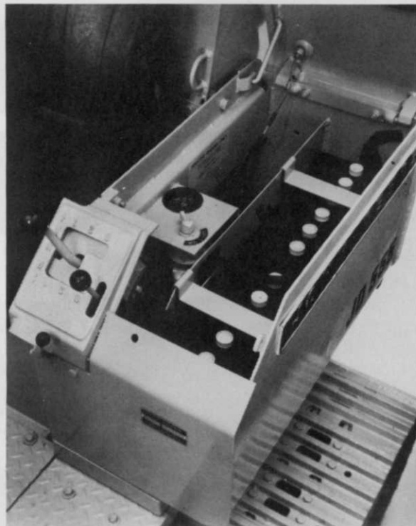
The heart of an electrical system in power equipment is the battery. It must be kept fully charged to provide maximum cranking power and prevent freezing of the battery solution.
