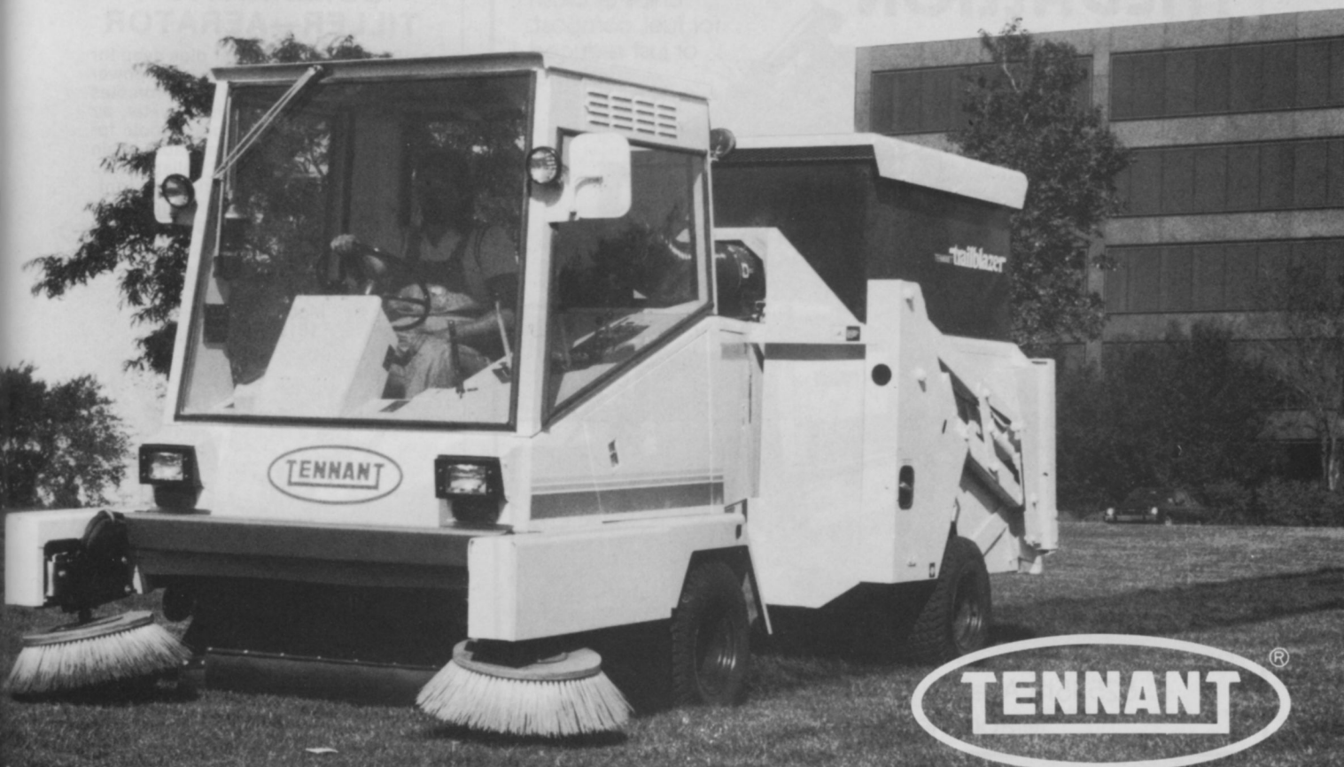
Cleans turf, hard surfaces. Climbs curbs to sweep hard-to-reach areas.
