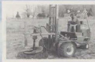
Hydraulic hole digger
