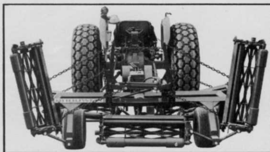
Brouwer 5 gang hydraulic lift P.T.O. mowers offer all standard Brouwer mower features plus hydraulic lift.
