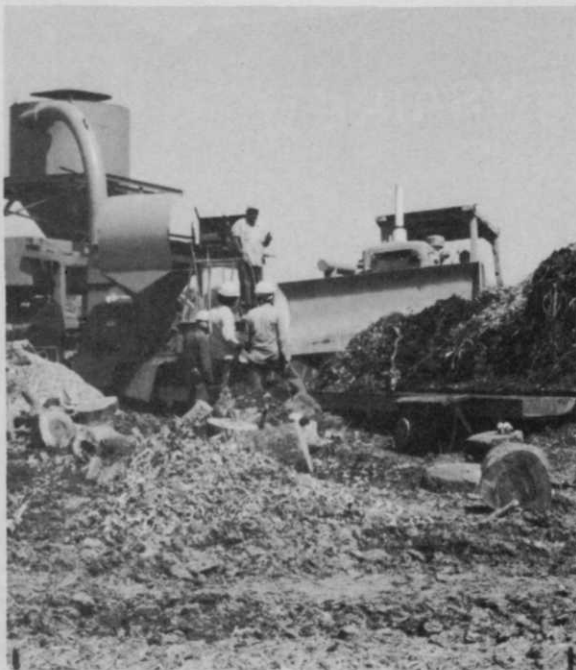
Large stumps and branches as well as chips made in the field are rechipped to achieve the right size particle for energy use.
