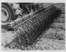
rows without adjustment. Its 3-point hitch matches category II, III, and most quick couplers. A safety shield offers operator protection. Yetter Manufacturing Co. makes it.
