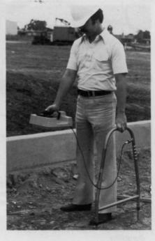
The device locates cables and gauges their depth. Then any damaged section can be found by following the cable and watching the meter.
