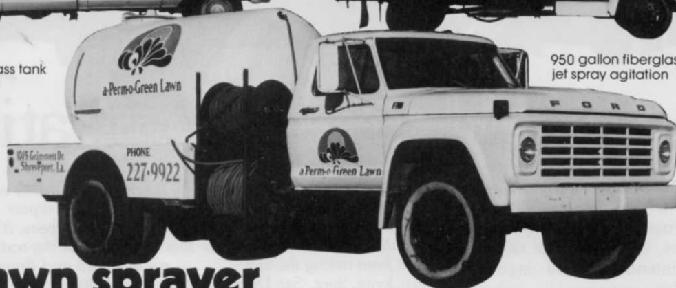
1,300 gallons all fiberglass tank and bed construction. (no rust or corrosion)
