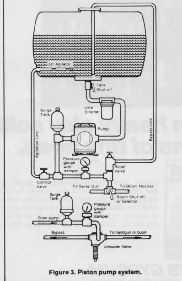
Figure 3. Piston pump system.
