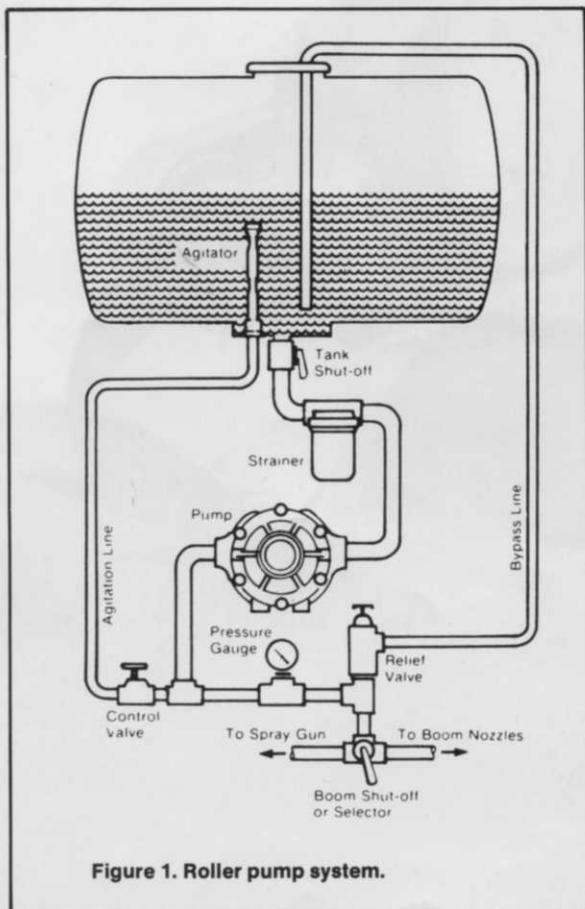
Figure 1. Roller pump system.
