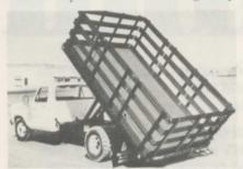
Works, Inc. body has 14-gauge steel stakes and a 12-foot-long platform of 100-percent, pressure-treated wood. Stakes are reinforced at their base with steel panel at and above the floor line.
