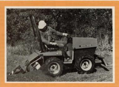
This little 18-HP-class trencher has a unique design which locks all four wheels into equal drive at the push of a pedal. Ground drive is hydrostatic...same as our big R100 model. A pedal-engaged master clutch permits quick cold-engine starts and will disengage all functions.
