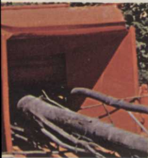
Positive Control feed rolls with instant reverse drive.
