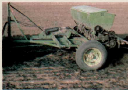
3. Grassland drills are an economical way of reestablishment of the seed crop. This can only be done if the fields are burned to get rid of the straw. Drilling is a one-step process putting down both seed and fertilizer.
