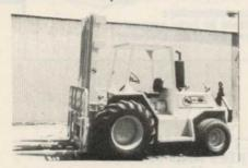
frame and body, and torque converter with power reversing transmission. Standard equipment includes side shifter, full time power steering, disc brakes, differential lock, overhead guard, work lights, and load backrest.
