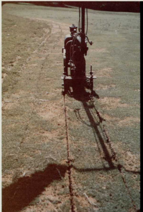
Examples of inventiveness. Power splitter for sods invented by Bill Lyons of Canal Fulton, Ohio (left). Two-man spiker circa 1939 (top right). Sprig planter from John Deere circa 1950 (bottom right). Photos by F. V. Grau.
