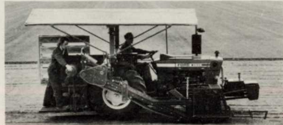
Model 2000 is the newest Brouwer harvester featuring automatic steering and empty pallet loading (top). Model A harvester is used by more sod producers than any other harvester.
