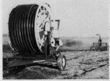
underground irrigation systems. The Nu-Way irrigation units carry up to 835 ft. of hose and are available with water turbine or gasoline engine power.
