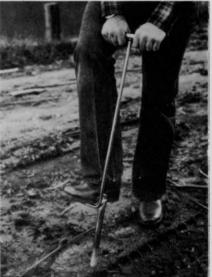
plated steel, the device is a onepiece unit with interchangeable tips for different soil types and conditions. A foot step eliminates stooping to insert the probe. Sample is removed by turning unit upside down.
