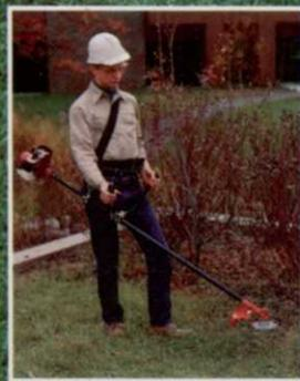
grass, weeds and brush. It's easily maneuverable with an adjustable U-handle control and wide strap harness for operator comfort.
