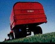
Wide track design, long wheel base and flotation tires provide excellent stability, even when capacity loads are carried.
